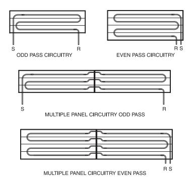
We provide design assistance. For assistance with complex applications or for in-depth information regarding radiant panel system design please contact our technical services department. Job project drawings showing panel layouts and piping are available for each individual project.
